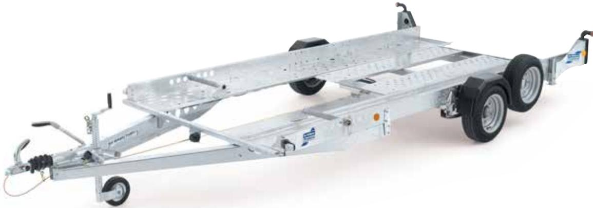
CT136TA twin axle with spare wheel and wheel chocks
